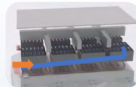
Upper/Lower Cover Sealing Foam for Battery PACK
